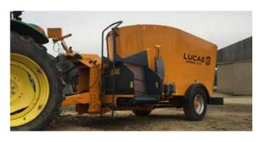
The SPIRMIX S diet feeders have been developed for farms where machine size is an important factor. These machines are compact and manoeuvrable. The rear axle is positioned to provide a very low overall height without compromising manouverability. The lowered machines are ideal for farms where the layout of buildings has height restrictions.
