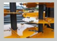
Vertical Rotors with spreading discs and superimposed projection trays to maximise efficiency and control the flow of straw.
