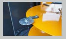
Cutting knives Mounted directly onto the discs they improve performance when using large round bales or highdensity bales.
