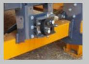
Male connector located at the frame of the bale spike. Allows you to control all the hydraulic functions of the machine without having to exit the telehandler.
