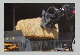
Suitable for handling round and square bales, equipped with 2 tines of 130 cm Ø 40 mm. 90 cm spacing between tines.
